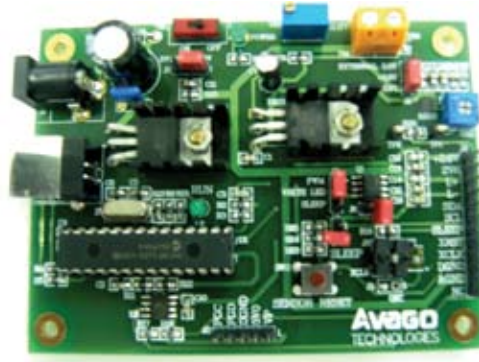
Figure 2. Digital Color Sensor Controller Board
